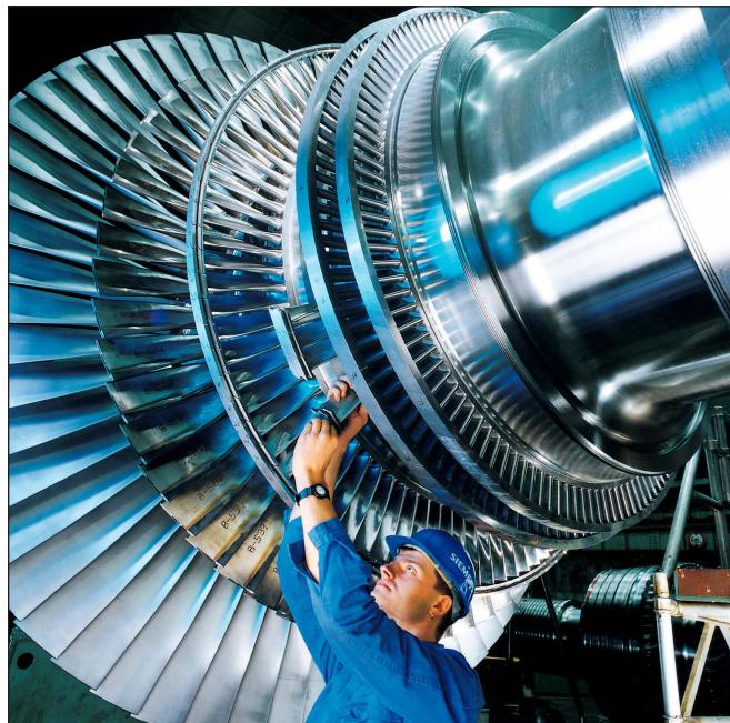
Rotor suvremene parne turbine (Izvor: [http://en.wikipedia.org/wiki/File:Dampfturbine\\_Laeufer01.jpg](http://en.wikipedia.org/wiki/File:Dampfturbine_Laeufer01.jpg))
